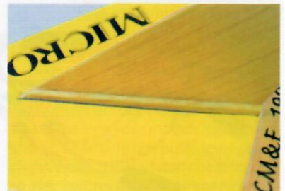
I modified the fin attachment with this additional piece of balsa.
