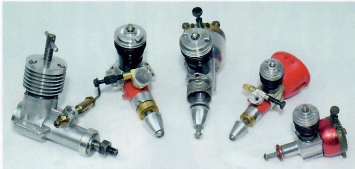
Suggested engines (L-R) - PAW 80, Cox TD, Cox Babe Bee (extended tank) for the Mini and Cox TD 020, Cox PeeWee 020 for the Micro.
