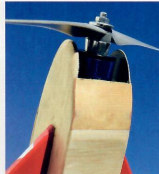
Adding the ply here reinforces the nose for less-than-perfect landings.
