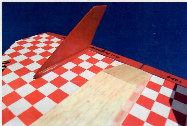
Fus, fin and elevons were all finished with sanding sealer. Colour was an additional coat of red then sealed with spray varnish.
