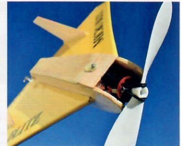
This is the most suitable method of prop retention when using small outrunners as it prevents bending the shaft when 'arriving' instead of landing.
