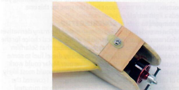
A simple hatch lock was fashioned from a piece of glassfibre sheet.
