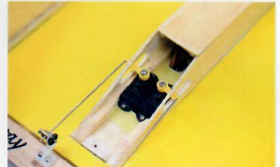
5g servos are more than adequate for the Micro Blitz. Two small pieces of thin fiberglass sheet glued to the balsa provided an anchor point for the screws.
