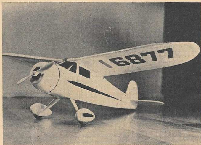
Sheet balsa sides with few simple bulkheads in fuselage; sparless wing almost falls together. Be sure to balance where shown.
