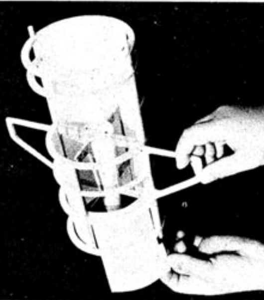
The 1/64 inch thick balsa liners are cut to fit, sanded smooth as shown, cemented in position.
