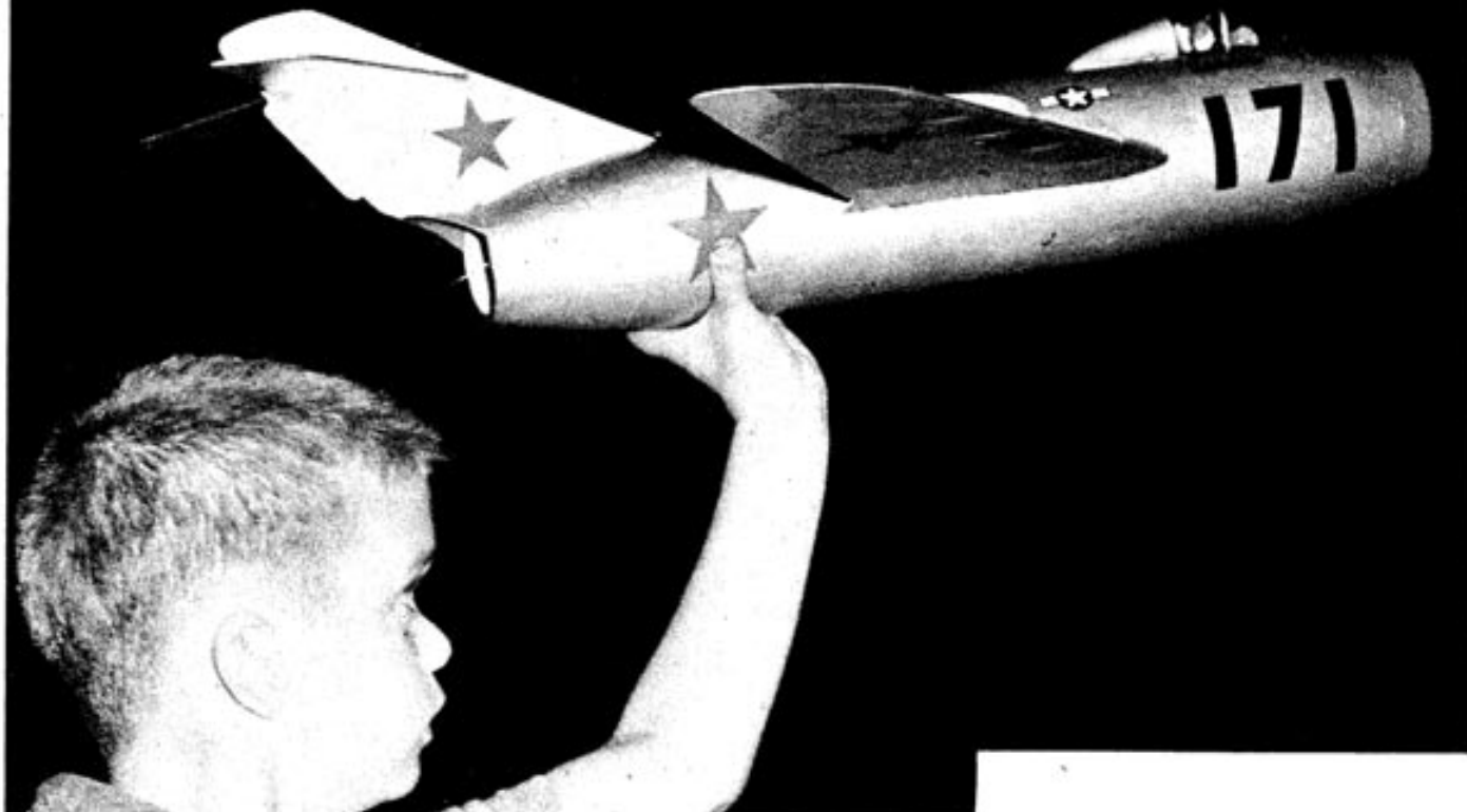
Proper method of hand-launching is demonstrated by author's son. Wash-out at tips is clearly shown.
