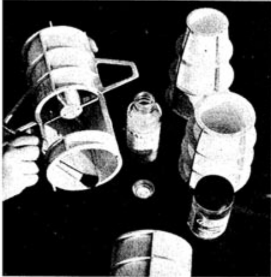
Nose, aft, sections lined Art Paper. With mid-body, one sealer, three fuelproof dope coats.
