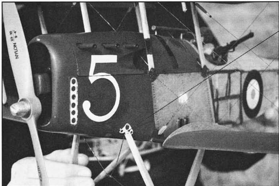
This close-up shows some of the details and that elephant marking. We see the trusty Mills 1.3, which used to belong to Eric Coates, is on a 9X4 Graupner.
