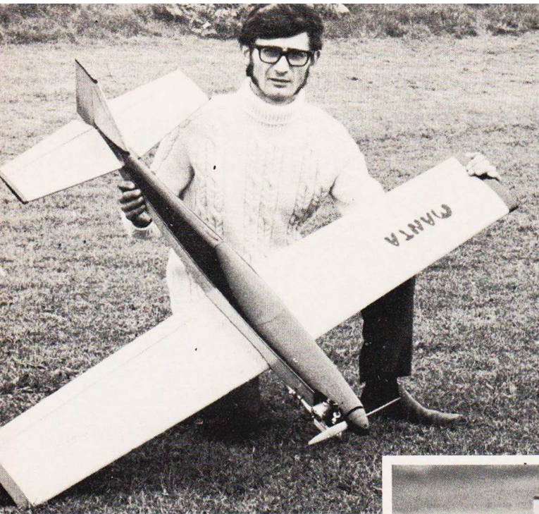
Left: designer Pat Ingrouille and prototype Manta. With a good .40 motor up in front, the aerobatic performance is excellent. Below: clean and simple, the straight lines of the airframe aid speed of construction.
