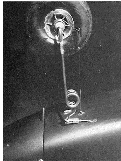
Wing hold-down dowels and nylon horn fairlead on elevator pushrod.
