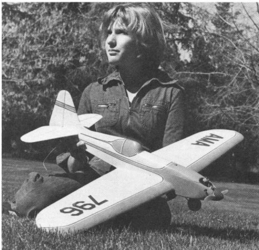
Miss Allison Carter shows off the classic lines of the "Madman". While the .049 TD is tiny in comparison with the original Orwick, the 1/2A model has adequate power.
