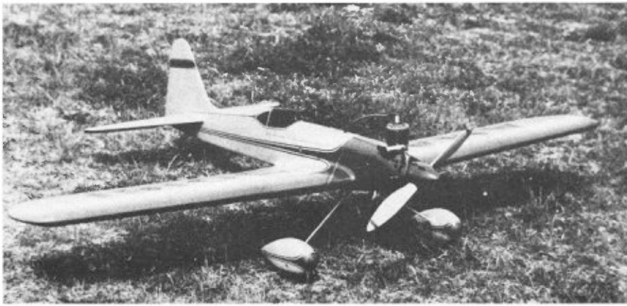
The original "Madman", built by J.C. Yates. Wheel pants were later discarded. Note the heavy ignition wire to the spark plug.
