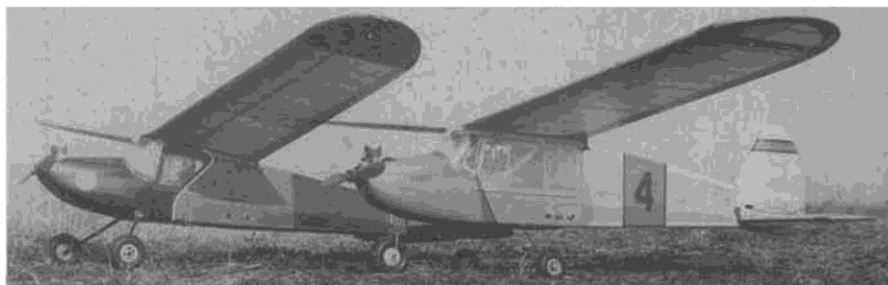
The Radart and Robot appeared to be fairly similar except for the landing gear. Nose wheel was always first thing to touch ground, even on better landings.
