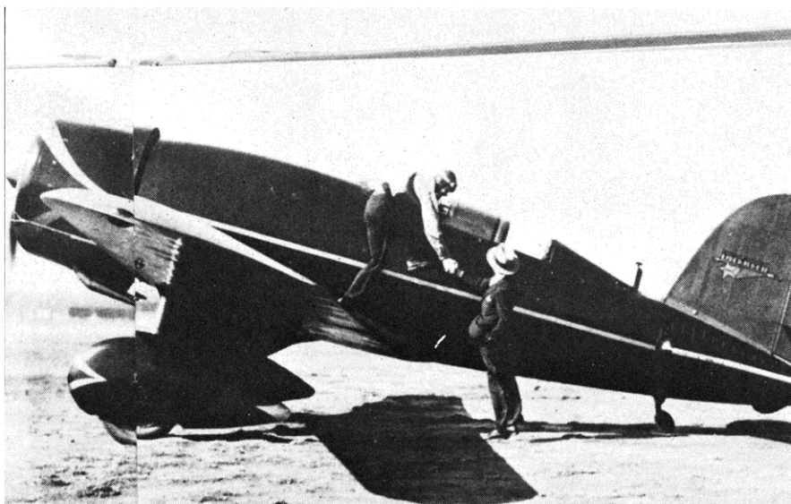
The Lockheed "Sirius" was designed by Charles Lindbergh, using components from previous Lockheed aircraft.
