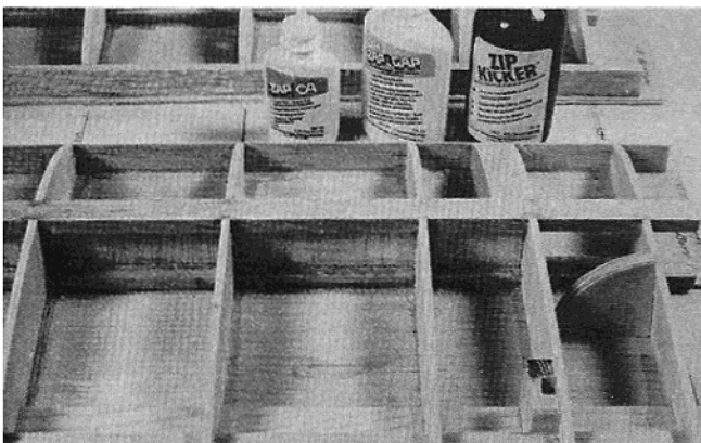
Inboard wing panel in early assembly stage. Note dihedral gauge for center rib.
