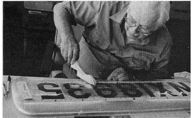
License numbers were cut from red MonoKote. Masking tape was used for location and alignment of numbers.
