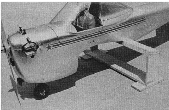
A simple stand bolted into wing mounting blocks is useful for safely transporting Little Dipper.
