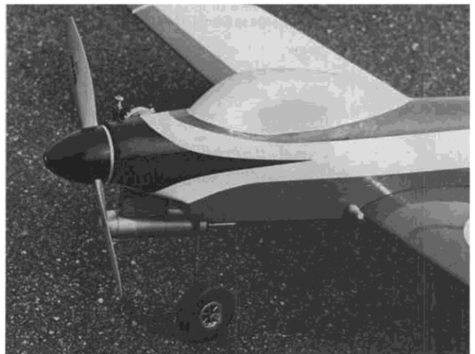
Side-mounted engine with nose faired into 2 inch diameter spinner. Stepped fuselage profile permits proper alignment.
