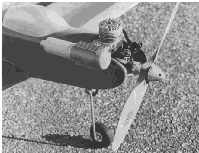
The so-called "quick and dirty" nose, with upright engine and open cowl. Requires higher tank location for proper fuel feed.
