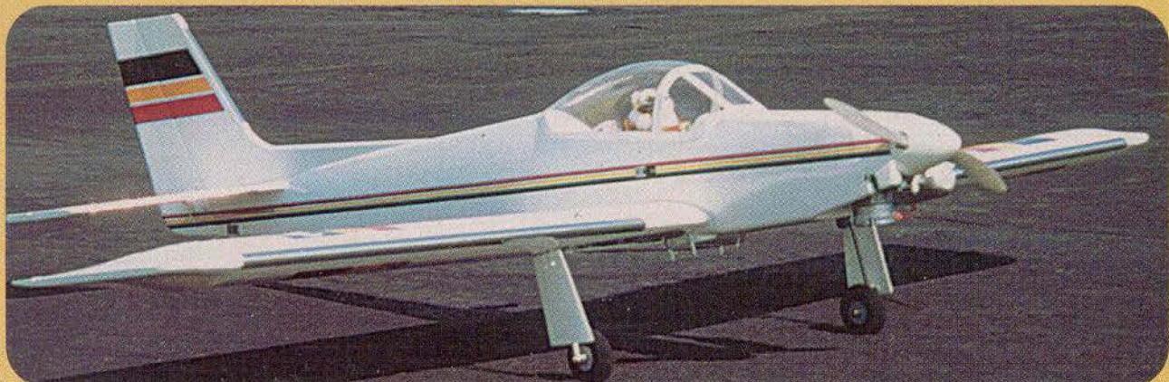
Prototype ready for take-off. White pegs under wings are the hinges for the inner gear doors, which were removed for the first flights. Note how well the engine is hidden in the partial cowling.
