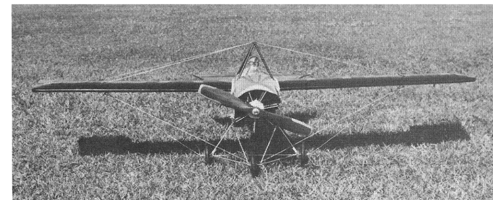
Al gives us a look at the landing gear set-up. Note the placement of the flying wires. A front view also gives us a look at the non-functional flying wire arrangement (below). A scale pilot and prop help the illusion (opposite page top). From a side view the dummy engine can be seen (opposite page bottom).
