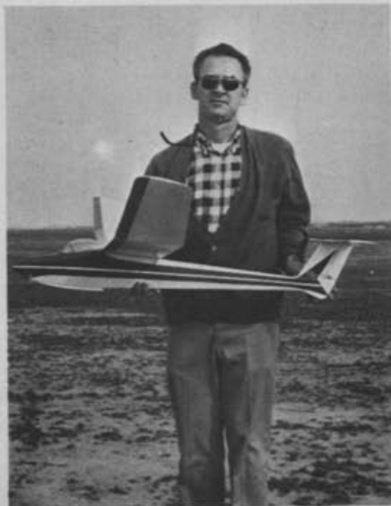
Nose to the grindstone. (Ooooh, that's awful!) Fuselage balanced to display inner space area. Servo installation comes next, then top sheet.
