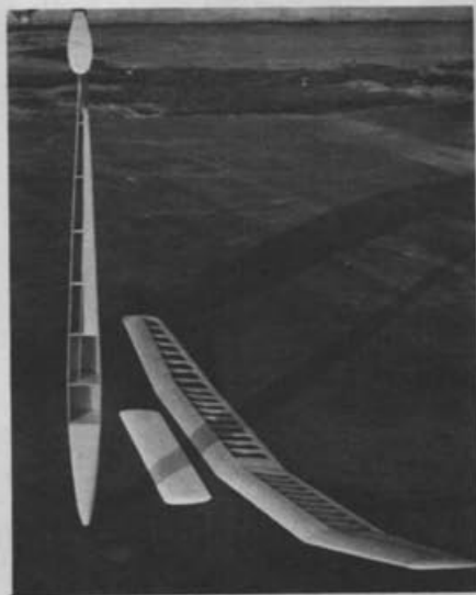
Nose to the grindstone. (Ooooh, that's awful!) Fuselage balanced to display inner space area. Servo installation comes next, then top sheet.
