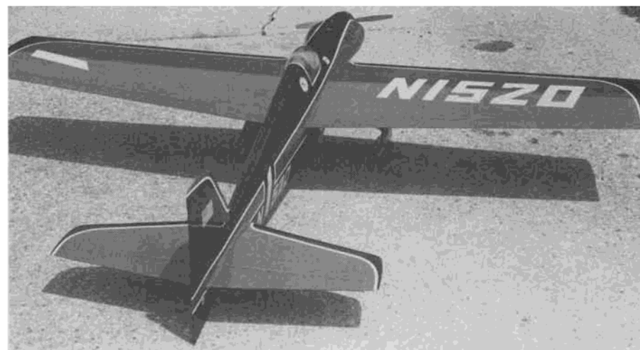
Although the wing is larger than on most Form I models, there is less drag and more lift, which keeps the model from "sliding out" and losing speed in turns. Uses stressed skin construction.
