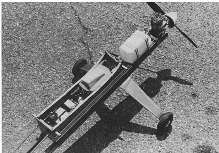
All sheet tail surfaces are held in place with two screws and a plywood clamp-alignment guide. BELOW: View of the radio installation.
