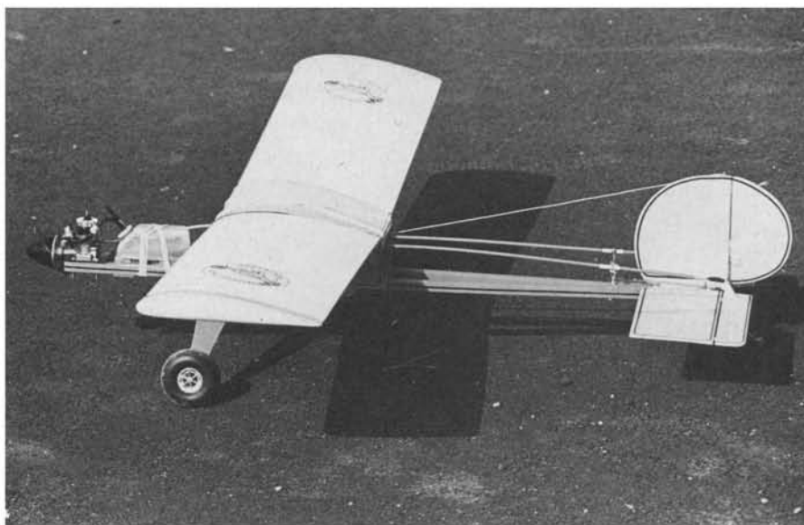
The Kwik-Stick III used a Jr. Box fly wing and O.S. .15 or .19. All-up weight, 3 pounds. Use innermost holes on short control horns for some real fun!
