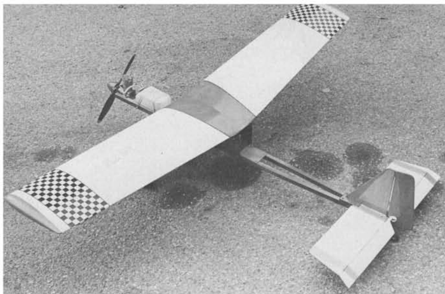
The Kwik-Stick II uses a Senior Box Fly plastic covered foam wing and O.S. .35 Gold 'N Rods not installed in this view.
