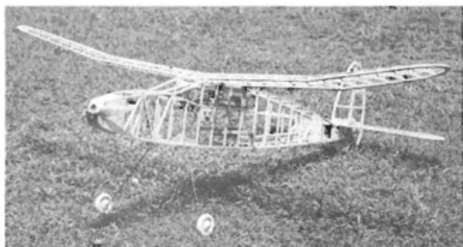
LEFT: Completed framework, ready for covering. Note that all equipment is installed prior to covering. RIGHT: An air intake gap is left between the leading edge and the fuselage, providing additional cooling air for batteries.
