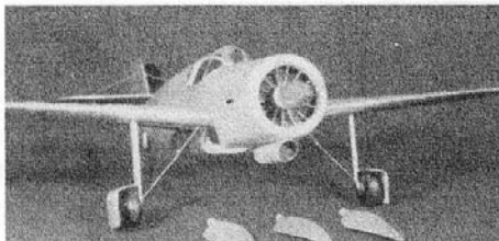
A real flying scale, if ever there was one. Note push-rods, oil-cooler tunnel beneath cowl and workable retracting landing gear.
