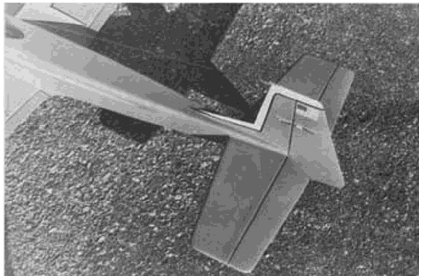
Rear section of Kaos shows how rudder area was increased over its predecessors.
