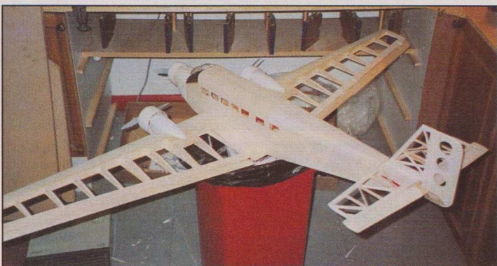
Top :George uses his own versatile fuselage jig for accuracy and speed. Wing construction shows capped ribs, servo housings and ply motor mounts. Cowling aligned for screw hole drilling. Note sloping battery tray aiming pack out through canopy in event of an arrival. Idea works well! Bottom :Completed airframe. Note gap between flaps/ailerons and underside of wings.
