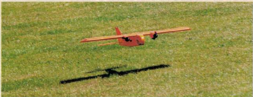
Not only is the electric version user-friendly in terms of launching, the shoulder wing underslung engine configuration makes it a doddle to land too!
