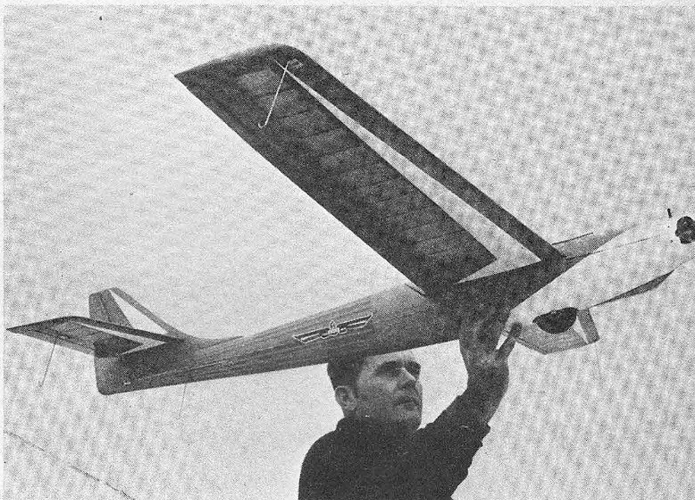
A clean, low drag configuration. Ship climbs at an amazing rate. 9/1 aspect ratio, wing withstands loops, it's mildly acrobatic.
