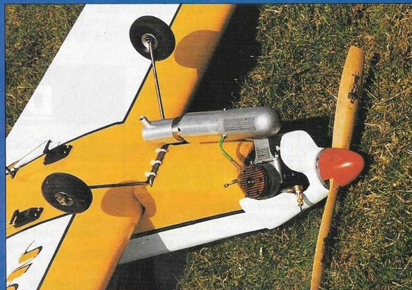
Innovation now has even more oomph thanks to an Irvine Q72. Nylon tie wraps provide a cheap and reliable way of retaining the undercart.
