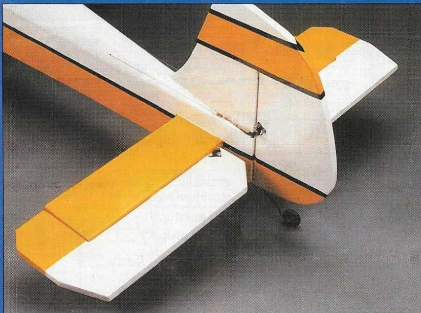
Tail surfaces are quick and easy to build from balsa. Note the squared off trailing edges.
