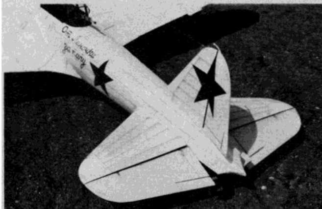
Large tail of Stormovik gives excellent low-speed stability and good ground-handling. Panel lines are Sharpie pen with airbrush shading.
