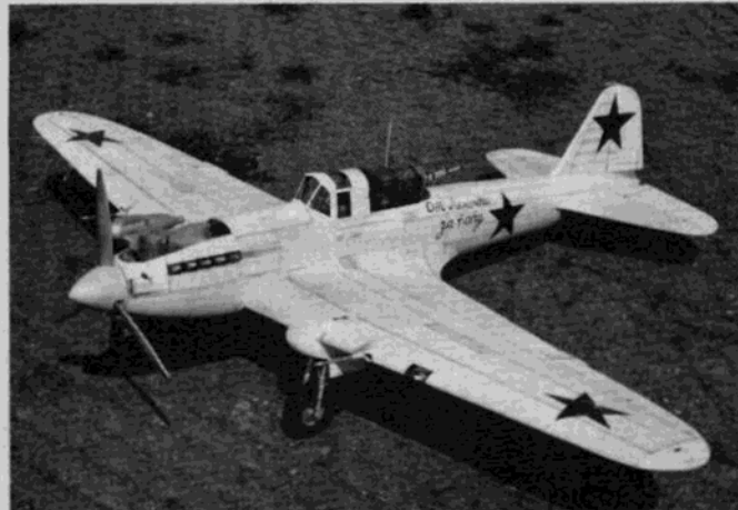
Stormovik is model of only truly armored aircraft. Not a fighter and not a bomber; it was designed to assault tanks at a very low altitude.
