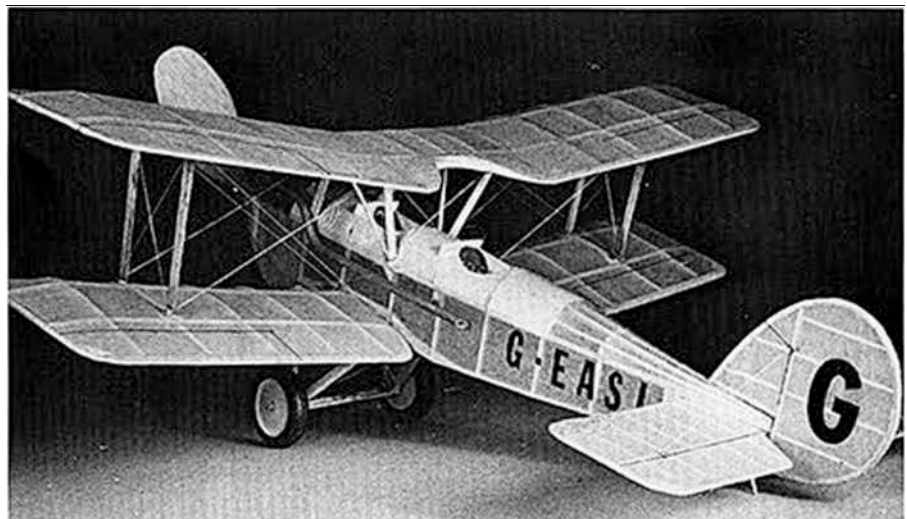
Beautiful little 13" span Boulton & Paul P-9, by Maj. E.F. Heyn(Ret). Wheels were heat-formed from acetate sheet. Power is a loop of 4mm Filati rubber.
