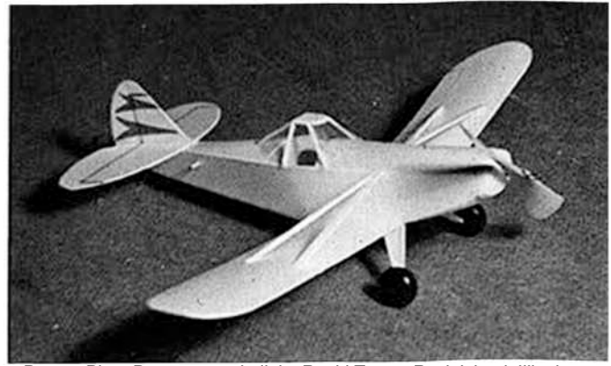
Peanut Piper Pawnee was built by Roald Tweet, Rock Island, Illinois, It's made entirely from sheet foam stock. Bag of Peanuts plan.
