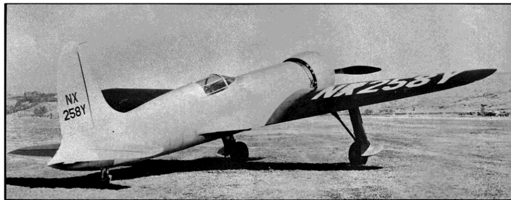
Detail on the landing gear brace and locking system can be seen in this three-quarter front view. Low pressure tires were required for a landing gear system which allowed for little shock absorbing.
