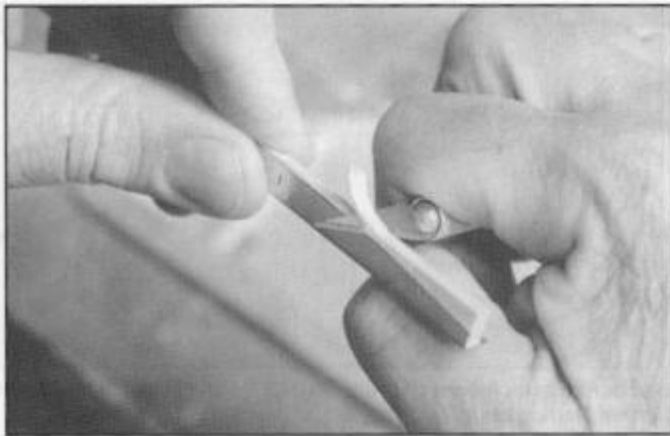
LEFT: Brass template used to cut stab ribs. Final sanding is done after assembly. RIGHT: Tail pattern is photocopied then transferred onto 1/16" balsa sheet. Assembled on flat surface. Details in text.
