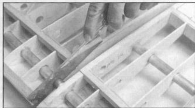
LEFT: Tip is beveled to match outer two ribs. Tested with straightedge before sheeting. Assures perfect alignment. RIGHT: Wing tubes are cut after mating wings.
