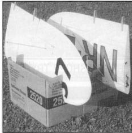
Cardboard box carrying case for wings. Prevents damage to wing wires while in transit.
