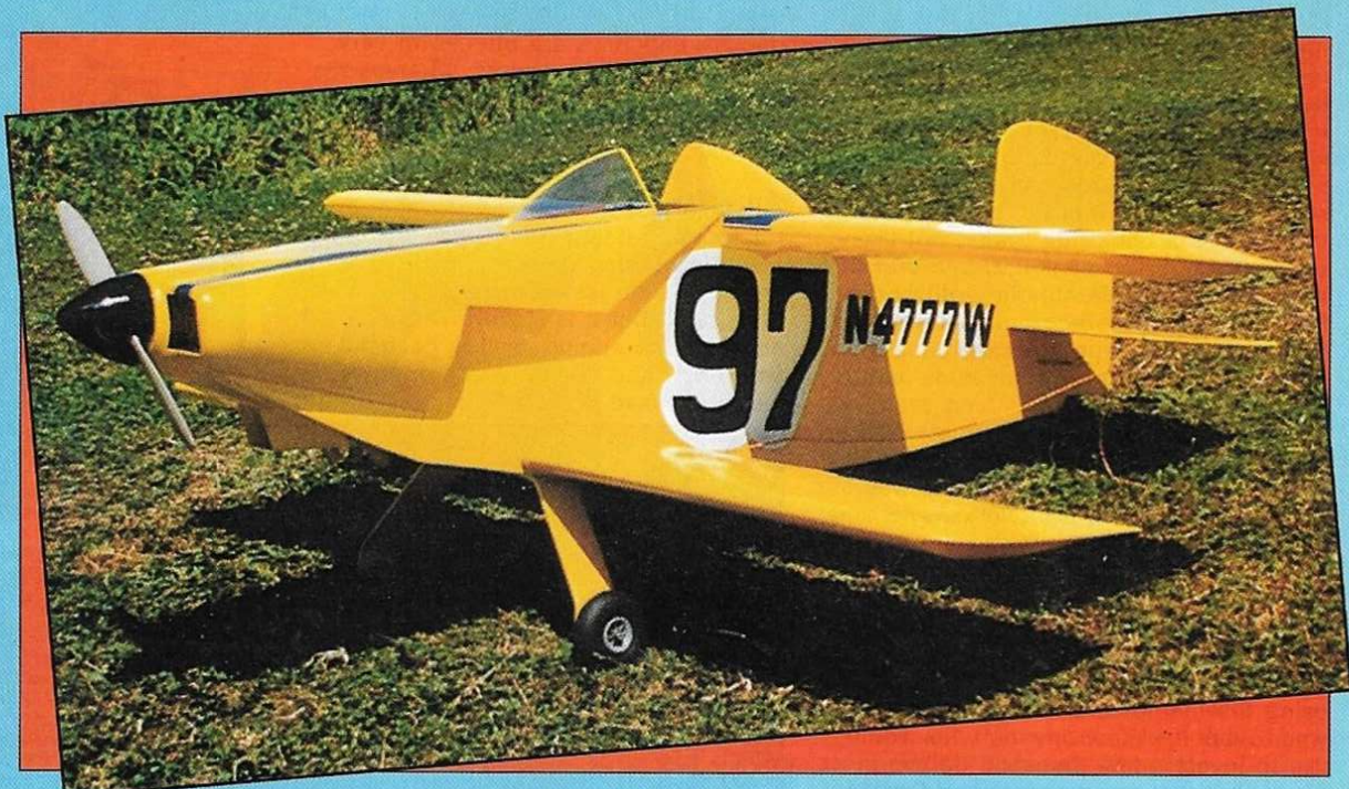
Hot Canary spans one metre – and is 1100mm long. Original was powered by an OS 46 SF ABC.
