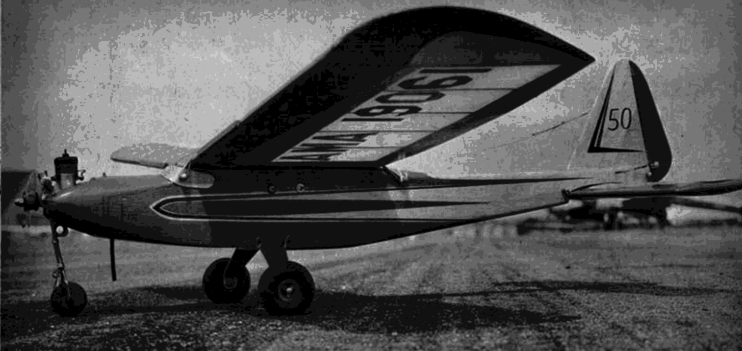
Hi-Fin with Fox .25 installation and 'Sunday-flier' rudder/fin combination. Also the wing, with flat tip plates, is shown in this photograph.
