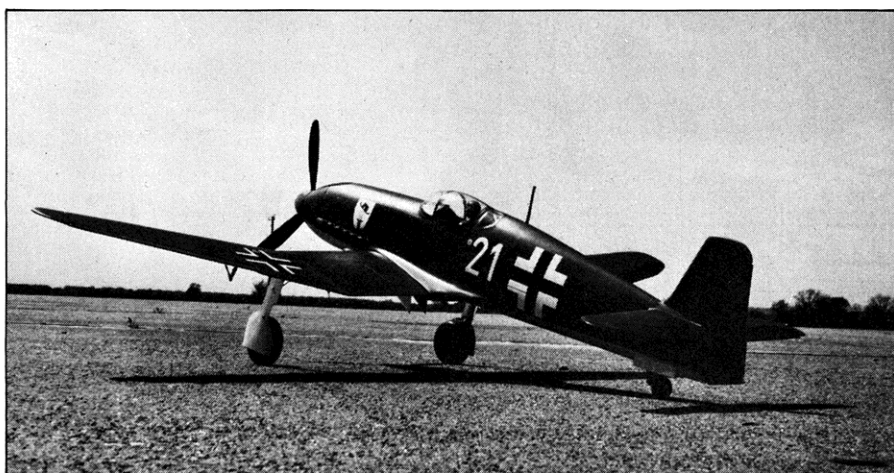
The wing has a slight inverted gull to it, which helps to keep the gear struts short.
