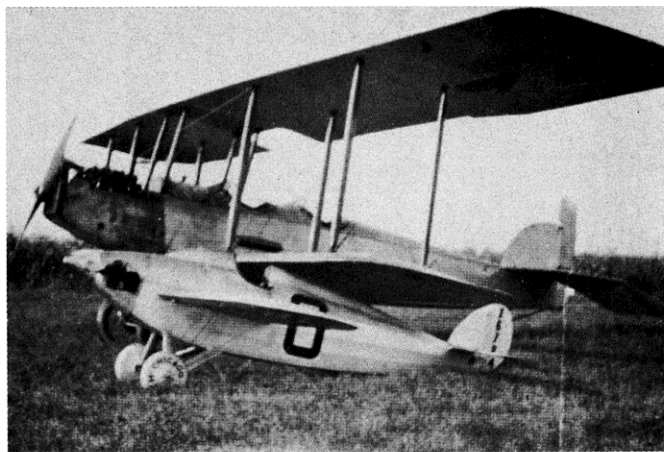
The tiny racing plane had a span of 16 feet and a Bristol Cherub engine for power. ▲
