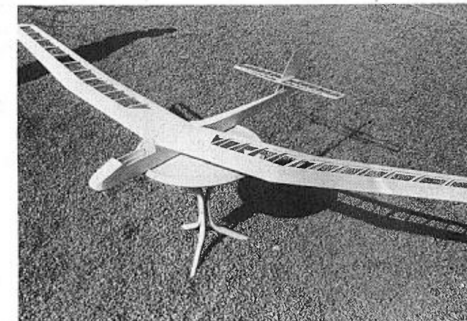
The completed Happy Face, ready for covering. Rugged, light, and easy-to-build.
