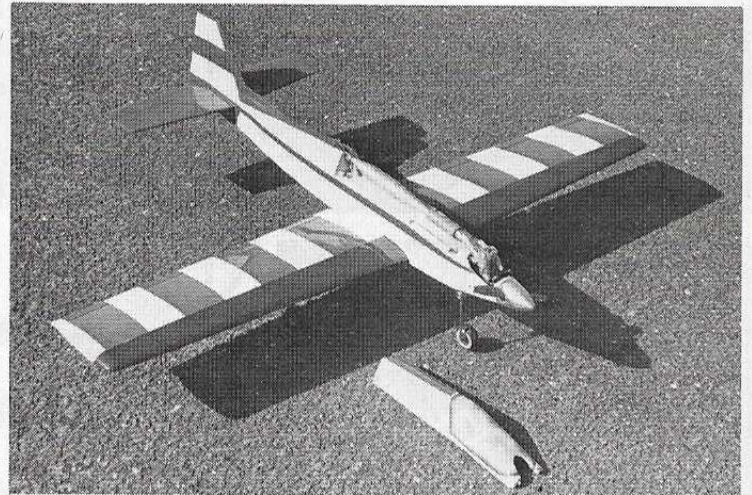
This is the optional, enclosed pipe version of the Hammer with the turtle deck removed to show actual set-up. Not much extra effort needed.
