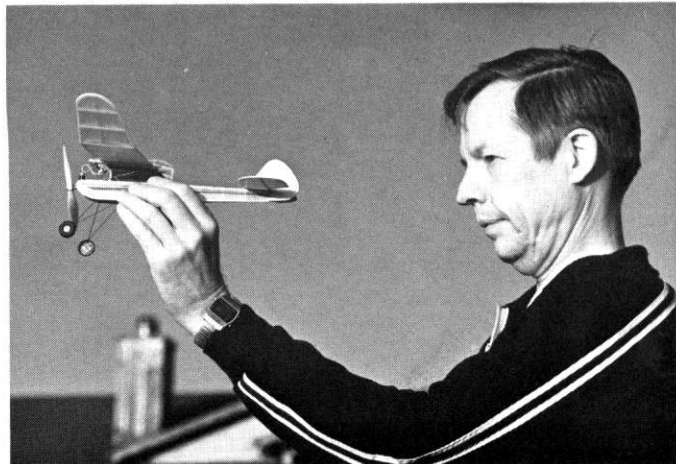
Weights engineer D. Dodgen admires lightweight Gym Dandy; liberal use of sandpaper brings down total weight considerably.
