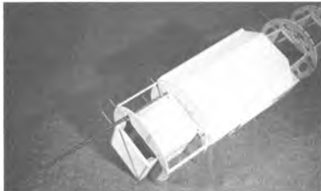
Drill holes for upper wing hold-down dowels.
