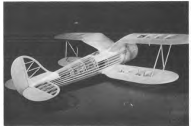
Gull Wing Bipe framed up and ready to cover.
