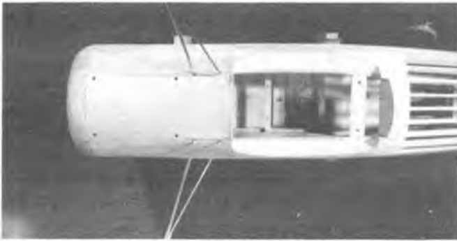
Landing gear installed with hatch bolted down. Note rear stringers are installed.
