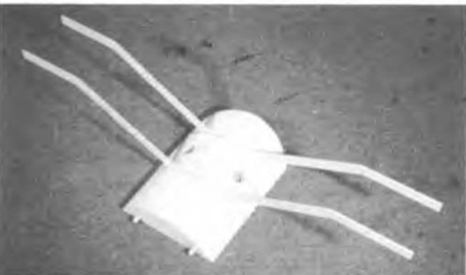
Medium hard balsa blocks contoured to fuselage. Holes are for servo leads.
