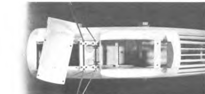
Bottom of fuselage with hatch removed. Gives access to L/G retainers and fuel tank.
