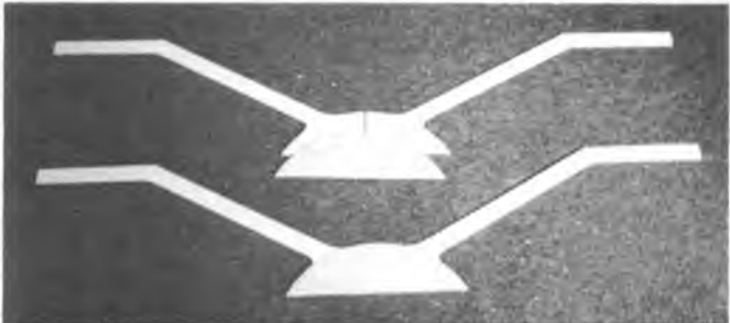
Top wing Gull center section — ply spars cut to shape.
