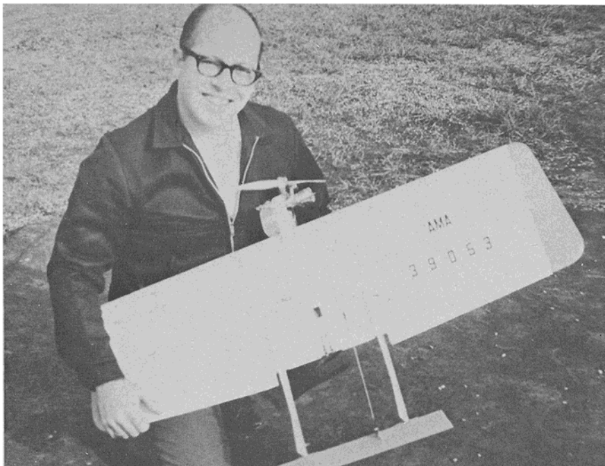
Little rudder area needed, yet Guillotine tracks well, won't spin, and is quite stable.
