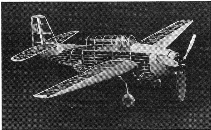
Structure is light and strong; ship convertible to small R/C.
