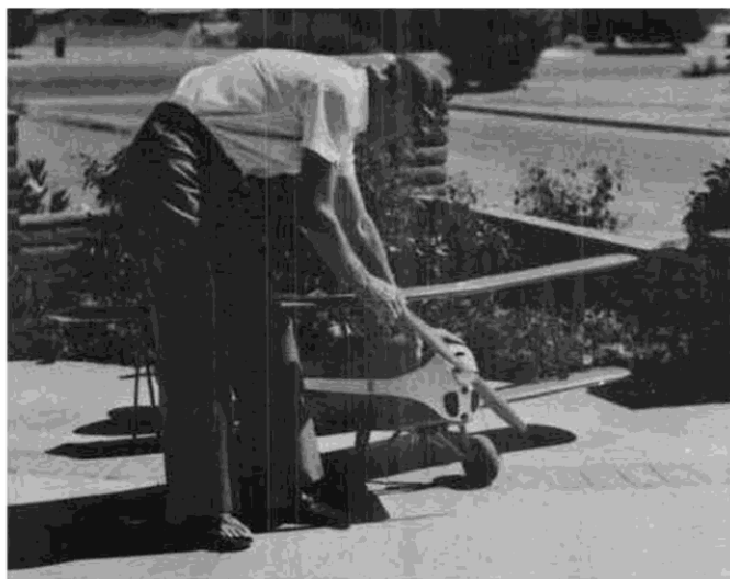
Frank shows how he safely turns the prop for pull-starting the Evra engine, from aside and behind.
