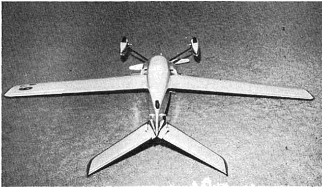
Bottom view detailing "V" tail pushrods and cooling vents at bottom side of wing.
