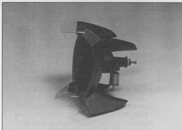
Front end of the fuselage is removable. Clear plastic vanes at the trailing edges of the cowl supports are the author's attempt to counter the torque from the CO 2 motor—explained in text.
