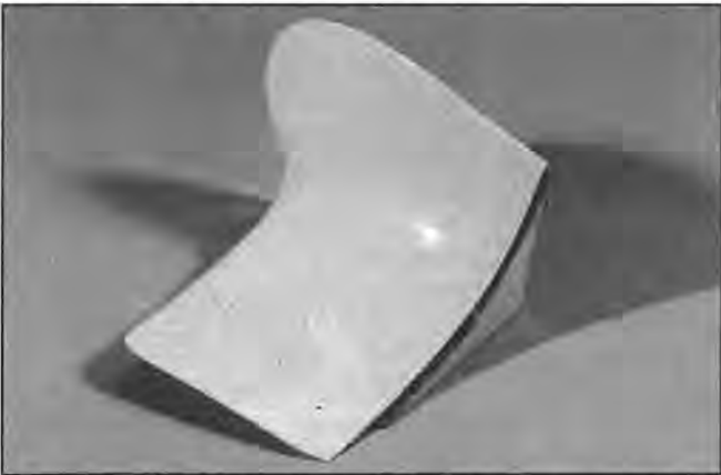
LEFT: If you glue WF4 to the plastic fillet front, you won't have to measure anything to get in the right place on the wing. Be sure to glue it only halfway across WF4 to leave a flange for the 1/16" sheeting. RIGHT: The fillet is sheeted with 1/16" balsa. The fillets were hammered out of aluminum by hand on the full-scale plane so you don't need to be too fussy here.
