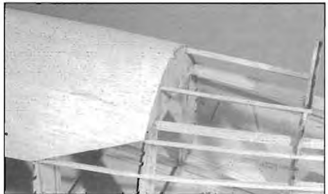
LEFT: The installation of the upper formers. The stringers for the top sheeting are also visible. RIGHT: The 3/32" top sheeting in place. Use 1/16" sheeting aft of F6.
