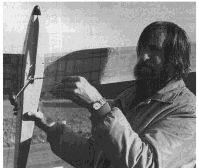
Pavel shows how the landing gear plugs into the fuselage; friction keeps it in place. Easily removed if necessary.
