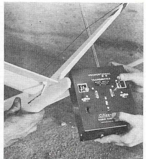
This shows left-rudder command — don't get your controls reversed. Both surfaces move up or down together for pitch control.
