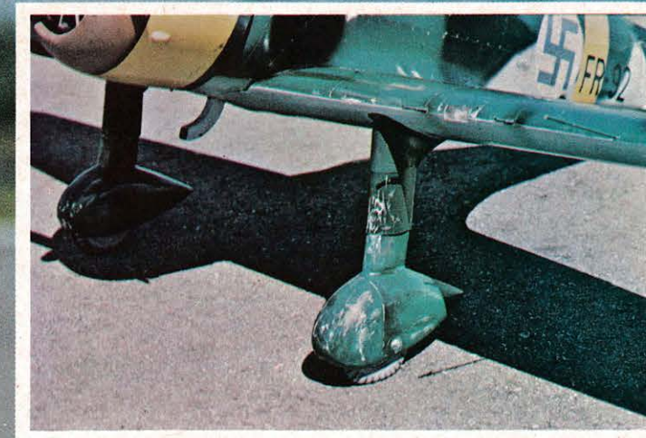
The long landing gear legs with their telescoping fairings make for an interesting stance on the long-legged fighter.
