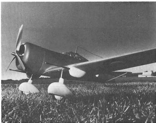
Danish model D.XXI showing details of the 20mm Madsen cannon gondolas beneath each wing. This particular model was fitted with a Cox Medallion .049 with throttle.
