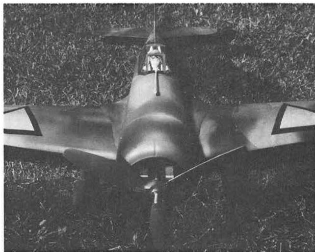
Frontal view of a Fokker D.XXI in Dutch Air Force markings illustrates minor differences in details such as gun sights and wheel pants.
