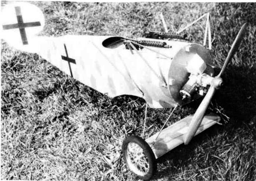
Close-up of fuselage reveals engine mounting. Guns are mounted on a removable hatch which gives access to the radio gear. All such stuff has to be well forward in this short-nosed design.
