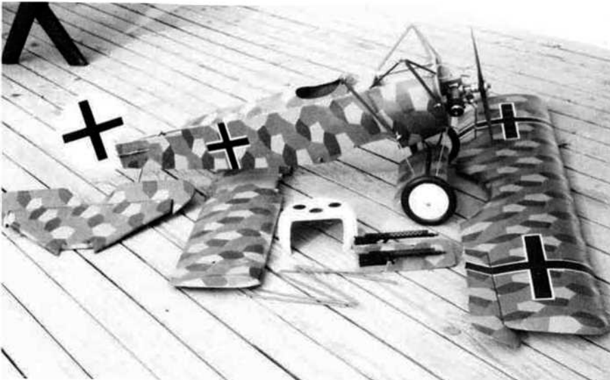
Close-up of fuselage reveals engine mounting. Guns are mounted on a removable hatch which gives access to the radio gear. All such stuff has to be well forward in this short-nosed design.
