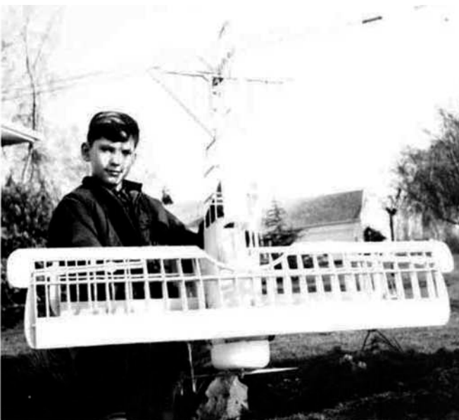
This picture, taken in 1968 (!) is of the author's son, Clark, holding up the bones of the D-VI for display. Construction was kept light.
