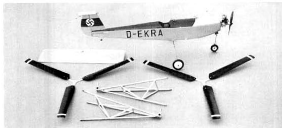
They haven't built a car small enough to make you leave this one home! If necessary, the main gear can also be removed in a couple of minutes. Three channels will do it all. A .35 for power.
