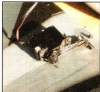
Short-coupled aileron servo sits centrally beneath wing.
