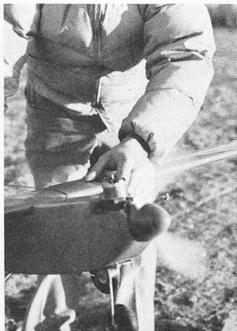
The Enya's idle is checked. Too fast and you're glued up in the sky until the fuel is consumed.
