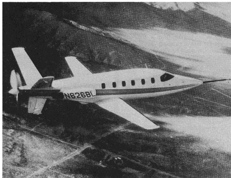
1981 aft fan by Lear — Lear Fan 2100. Two turbo-prop engines geared to a single propeller.
