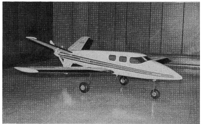
Firestreak finished and ready to fly. Graphics are MonoKote on MonoKote. Lettering and numbers are Rub-On transfers covered with clear MonoKote.
